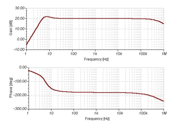
The noise response of the amplifier measured across the 10k load is shown below. Please note that this plot was made with the mic insert replaced by a signal generator.
